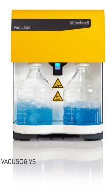
VACUSOG suction washer for the separation and neutralization of inorganic acid fumes created during Kjeldahl digestion. With integrated vacuum pump - No water supply is necessary.
