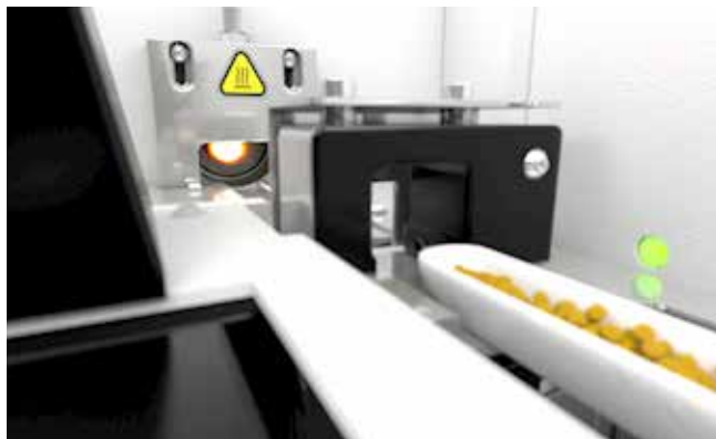
High temperature ceramics (HTC technology) for catalyst-free combustion at up to 1300 °C
