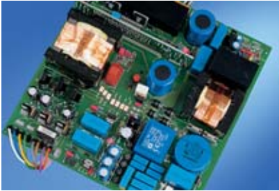
“Connect and disinfect” - electronic ballast for the ideal operation of the Spektrotherm® UV lamp
