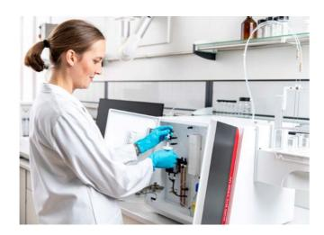
**Smooth workflows – just analyze**: Clever automation functions enable that additional samples can be reloaded without pausing the measurement process. When switching from automated liquid to solid analysis, no hardware conversion is necessary.
