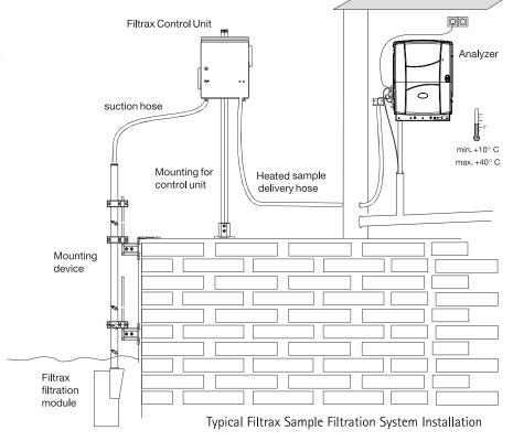
The Hach Filtrax Sample Filtration System module holder should be installed at least three inches from the bottom of the tank and must have between three and 18 inches of water above it. Mount the control unit on a wall with three #10 mounting screws (supplied). Four pipe bracket locations for vertical or horizontal guardrail mounting are provided. (All measurements at the right are in mm.)
