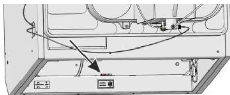
Fig. 6 Electrical connection for the heated transfer line
