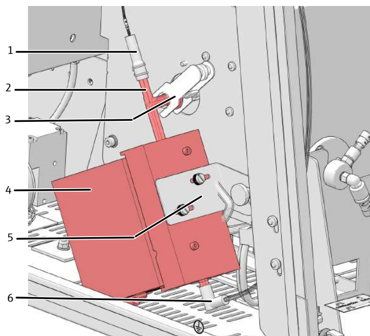
Fig. 12 Peltier cooling block with T-connector
