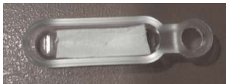
Fig. 24 Quartz boat with correctly inserted quartz fleece
